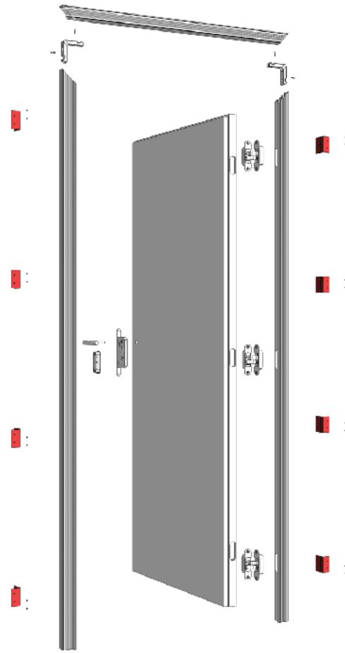
InSensation's FS2 Frameless Swing door is the easiest and strongest 2" thick frameless door to install. All the components, hinges, magnetic lock, leaf and frame are pre-milled and pre-installed in our manufacturing facility. This will save you hours and days of work.
