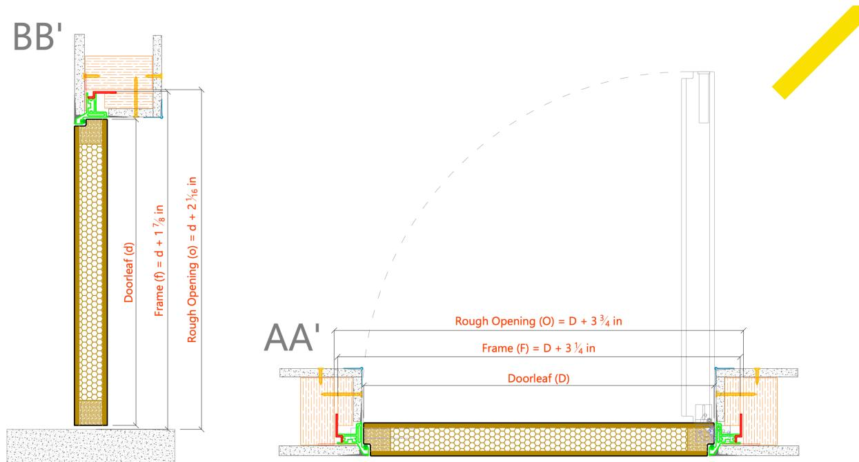
The Insensation FS doors are **universal** doors, meaning they can be installed either PULL-OUT or PUSH-IN using the same exact frame. Simply turn the frame 180° to change the function. The installation procedure remains identical in both instances.
