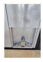
25 Using a 13mm socket, loosen the pin block retaining bolts at the top and bottom of the door.
