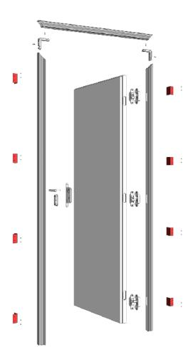
Insensation's FS1 Frameless Swing door is the easiest frameless door to install. All the components except the outer L-brackets are pre-milled and pre-installed in our manufacturing facility. This will save you hours and days of work.
