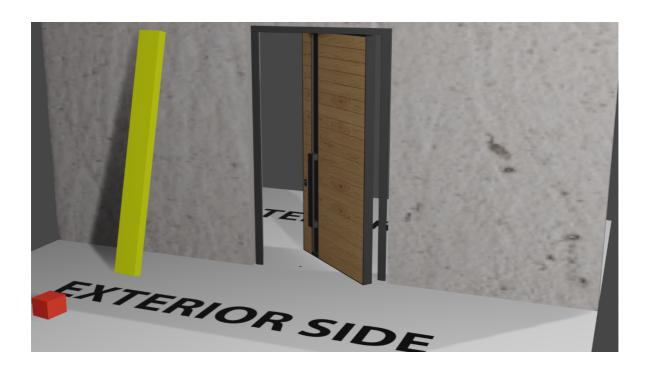
9) After installing the outside panel, install the inside panel and screw the perimetrical restraint profiles. (Usually, the upper and he bottom one are pre-installed making it easier to install the panels)
