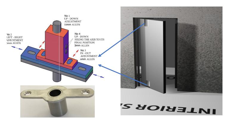
8) After fixing both hinges in their final position, it is time to install the panels. In some cases the exterior panel is already installed on the door. If this is not the case, start by installing the exterior panel on the door, using **neutral** glue between the metal core and the panel. WARNING! Using silicon glue or other acidic glues may result in color damage (especially on glass panels).
