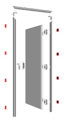
Insensation's FS1 Frameless Swing door is the easiest frameless door to install. All the components except the outer L-brackets are pre-milled and pre-installed in our manufacturing facility. This will save you hours and days of work.
