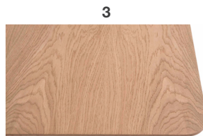
3 Veneered Oak, Vintage Oak and American Walnut on MDF E1 th. 40mm. Veneered border 10mm. Then shaped bevelled at 25°. Rounded corners.
